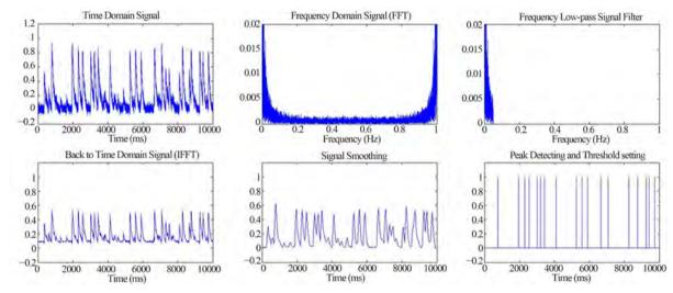
Figure 2. Neural activity signal processing. a) Original time series signals; b) FFT frequency signals; c) High frequency filter; d) IFFTtime series signals; e) Signal smooth process; f) Voltage threshold method of spiking detection.
